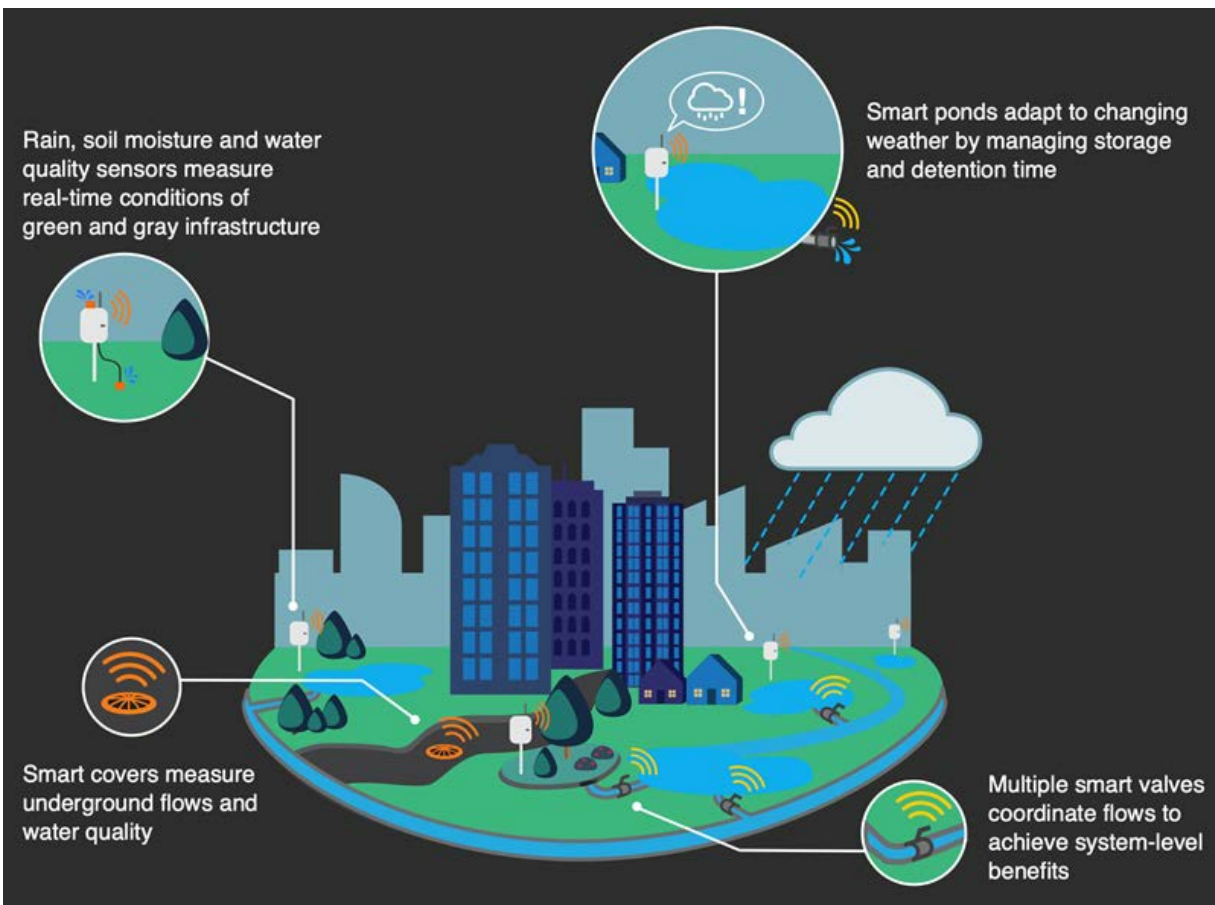
Figure 8. A graphic that depicts the variety of smart sensors and their uses in the Open-Storm project.
